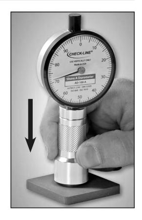
**IMPORTANT:** After the initial reading has been noted, continue maintaining pressure for several more seconds. Creep or cold-flow of the specimen, if present, will be evident by receding action of the dial hand.
