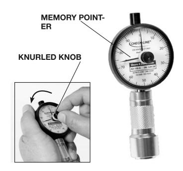
instrument counter- clockwise until the pointer has been reset.
