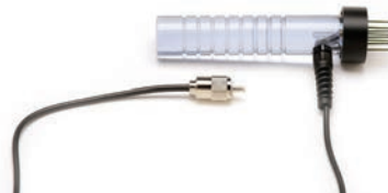
37-E/C - Used for yarn, 1 1/2" pins with 1" penetration
