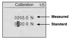
The current measured value should equal the standard force applied. If the values do not match, press "ZERO" and the "MODE" keys to correct the measured value. Press "MENU" to enter the next calibration point.
