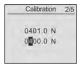
After any of the calibration points have been completed, touch "LOG" to exit the calibration mode. Then save the calibration or discard by pressing "Yes" or "No". After completing the calibration of the 5th point, the confirmation window will automatically ask to "Save and Exit" by selecting "Yes" or "No".
