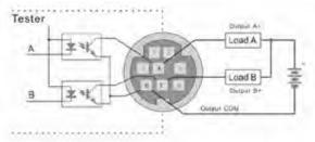
When the measured value is less than the lower limit tolerance value, the "pc2" operates, 7pin and 6pin line conduction. Whenthe measured value is more than the upper limit tolerance value or 110% of the rated capacity, the "pc1" operates, 4pin and 6pin line conduction.
