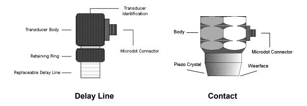
The Transducer is the "business end" of the *PZX1-DL*. It transmits and receives ultrasonic sound waves that the *PZX1-DL* uses to calculate the thickness of the material being measured. The transducer connects to the *PZX1-DL* using a single shielded coaxial cable with microdot connectors.
