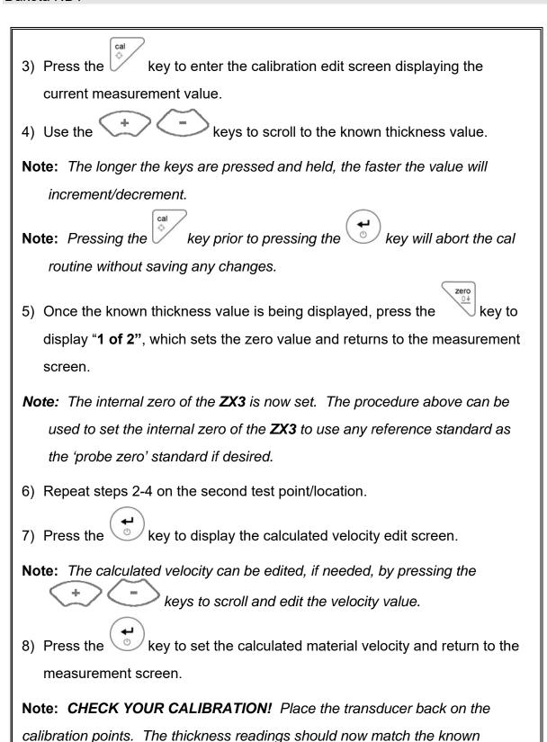
thickness values with minimal error. If the thicknesses are not correct, repeat the steps above.
