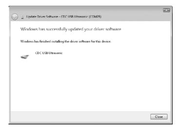
Open device manager again to reference the communications port assigned to the CDC device, it will be displayed to the right of the CDC device. Now that the driver has been successfully installed, a 'keyboard wedge' with serial communications capability can be used to connect to the ZX-6 and will capture the measurements to your PC when the ENTER key is pressed:
