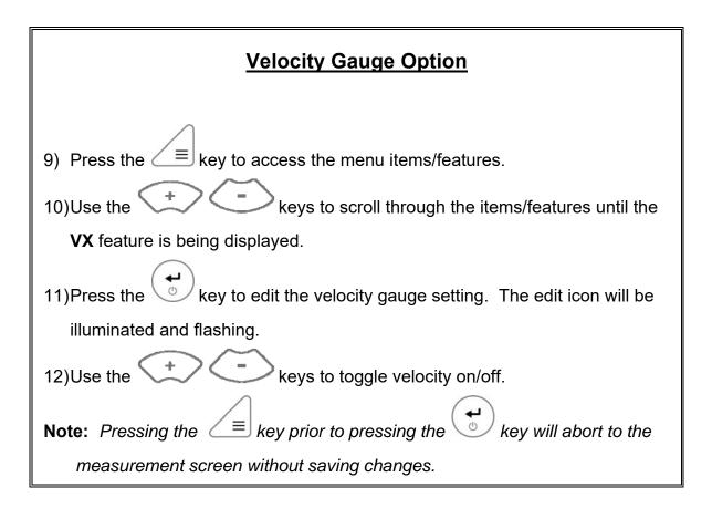
13)When the desired **VX** setting is displayed, press the key to set the status and return to the measurement screen.
