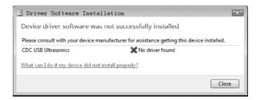
The driver file that needs to be installed can be found in the examples folder created on your PC by installing our DakView PC software, and is located in the USB folder. The file name is CDC\_Ultrasonics.inf.
