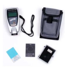
3000EZ Series gauges are supplied as a complete kit, with gauge, plastic calibration shim, 2x AAA batteries, soft carrying pouch, manual and manufacturer's calibration certificate.
